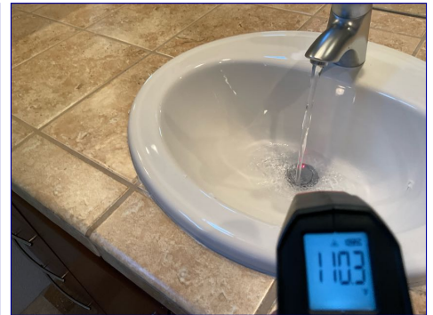
Water temperature test was good. Hot water.
