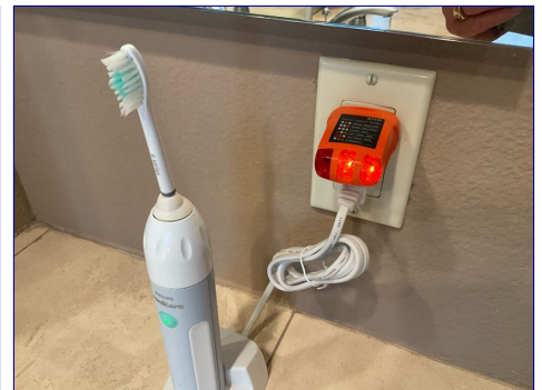
No reverse polarity or open ground. GFCI worked properly.
